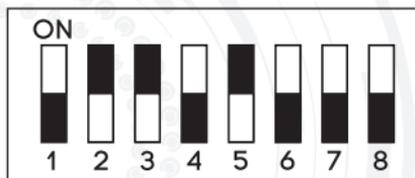
$$0 \times 2^0 + 1 \times 2^1 + 1 \times 2^2 + 0 \times 2^3 + 1 \times 2^4 + 0 \times 2^5 + 0 \times 2^6 + 0 \times 2^7 = 2 + 4 + 16 = 22$$
